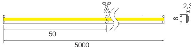
IP 20 | 24Vdc | -20°C / +40°C | 480 LED / m | IRC 90
