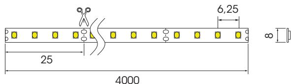
IP 20 | 24Vdc | -20°C / +50°C | 160 LED / m | IRC 90
